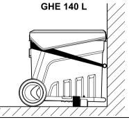
• Secure the machine against slipping using suitable fastening materials. Attach ropes or straps to wheel carrier (1) or feed chute (2).
