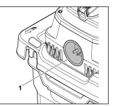
Connect the mains cable connector to mains plug (1).
